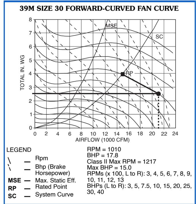
Airflow with a clean filter will be 21,000 cfm. Also note that the horsepower goes from 17.8 bhp to about 28 bhp because the FC fan is an overloading type fan.
