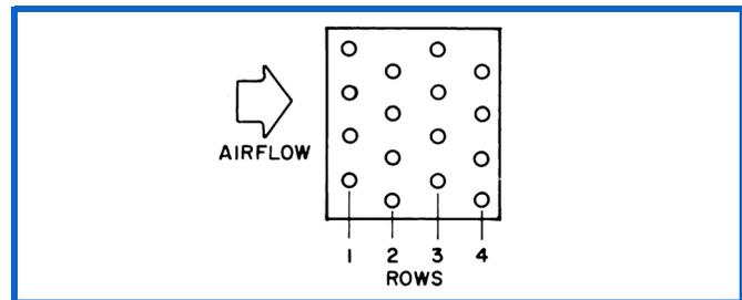
Cooling coils are typically available in 4, 6, 8, and 10-row configurations. Tubes should have an outside diameter (OD) of 1/2 in. to maximize heat transfer at minimum water flows. Coils should be sized for the most efficient use of water. Water temperature differences of 12 to 16° F are typical and represent optimum selection points.
