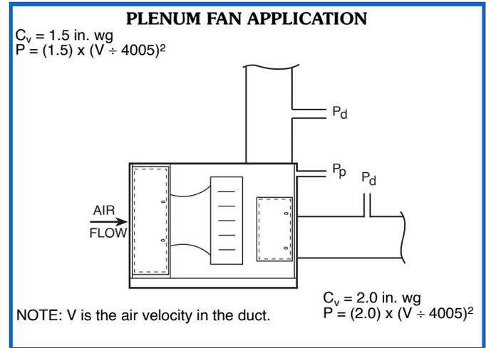
The 39M Series airfoil and forward-curved fans are tested as part of a system with straight discharge ductwork, and the fan ratings are based on this duct design. When designing ductwork in the field, it is important to use a straight discharge duct of the correct dimensions to obtain maximum fan performance. Straight ductwork helps the airflow to develop a uniform velocity profile as it exits the fan and allows the velocity pressure to recover into static pressure. See the figure below.
